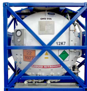
Rear view showing additional fill connection
