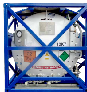
Rear view showing additional fill connection
